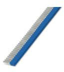
Ferrule, Dimensions according to DIN 46228-4, with color-coded plastic collars according to NF C 63-023:1994-02, for processing with the CRIMPFOX 4 in 1, sleeve length: 8 mm, color: blue, number of strips: 10, number of sleeves per strip: 50
