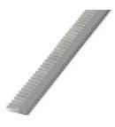
Taped ferrules, 0.75  $\rm mm^2$ , sleeve length 8 mm, with plastic collar, according to DIN 46228-4, gray, for processing with the CRIMPFOX 4 IN 1, 10 strips each with 50 sleeves per strip.
