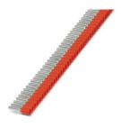
Taped ferrules,  $1.0 \text{ mm}^2$ , sleeve length 8 mm, with plastic collar, according to DIN 46228-4, red, for processing with the CRIMPFOX 4 IN 1, 10 strips each with 50 sleeves per strip.
