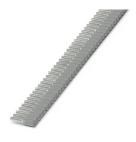
Ferrule, Dimensions according to DIN 46228-4, with color-coded plastic collars according to NF C 63-023:1994-02, for processing with the CRIMPFOX 4 in 1, sleeve length: 8 mm, color: gray, number of strips: 10, number of sleeves per strip: 40
